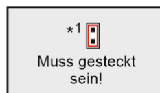
Jumper *1 for terminating the interface
