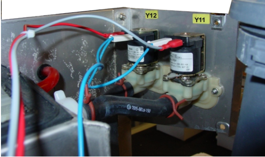
Y11 - Cold water valve (grey/blue cable) Y12 - Hot water valve (red/blue cable)
