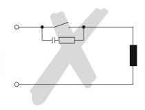
An RC filter should not be fitted directly to the regulator's switching contact (as shown on the left), as an idle current will flow through the RC combination even when the switching contact is open. This current may be enough to mean that a downstream contactor is not de-energised and a closed protective contact does not reopen.
