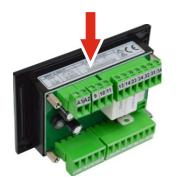
The correct circuit diagram for your controller is affixed to the housing and is also included in the Accompanying Device Documentation.
